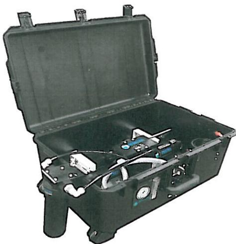
The system is encased in a military grade, shock resistant, non-corrosive case and powered by *any 24V DC source*. This system is so efficient that it can be run from a vehicle's electrical system, a solar panel, or battery bank.
